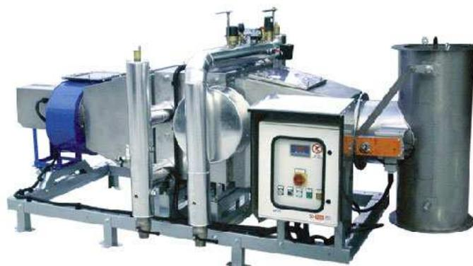
Realization of heat recovery units from heat sources with emissions into the atmosphere, by transformation into hot fluids
